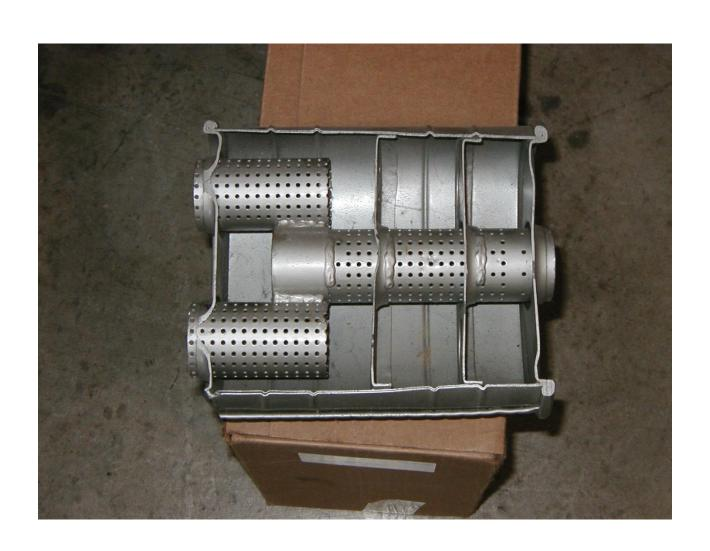
My added flow Tubes with wall separators and washer to reduce the inner exhaust tube harmonic pulse.
