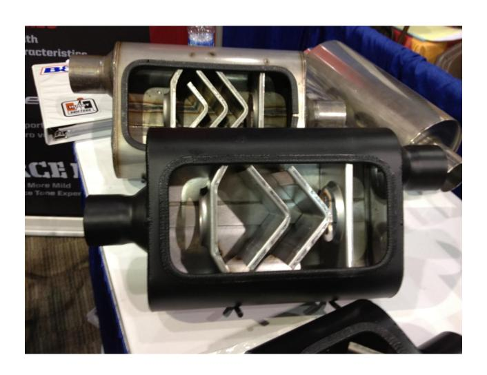
Frequency tuning is used to cancel the exhaust flow resonance at the 2000 rpm. The washer welded on the shorter outlet helps reduce the wave resonance. A further reduction can be achieved by running a tube from the inlet to one totally exclusive outlet.
